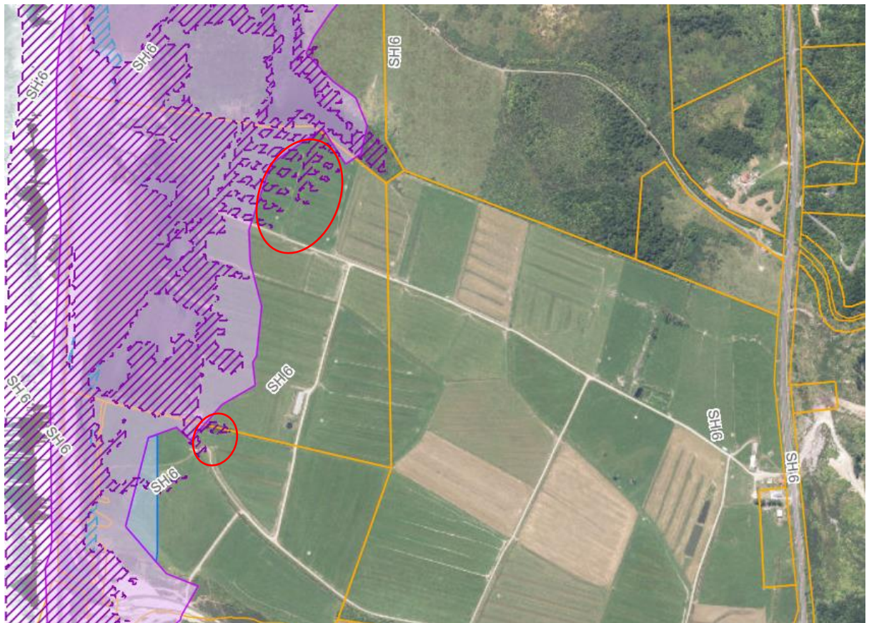
Figure 4– The updated LiDAR flood hazard model illustrated in the Draft variation to the TTPP. The red ovals indicate the areas of draft coastal alert areas that are in addition to that indicated in the TTPP.
